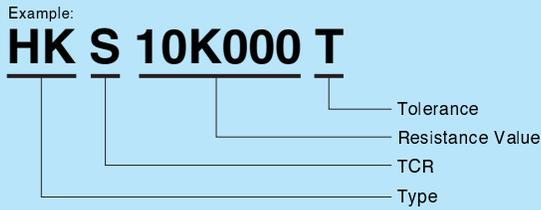
Resistance value, in ohm, is expressed by a series of six characters, five of which represent significant digits. The sixth R or K is a dual-purpose letter that designates both the value range (R for ohmic; K for kilo-ohm) and the location of decimal point.
