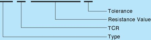
Resistance value, in ohm, is expressed by a series of six characters, five of which represent significant digits. The sixth R or K is a dual-purpose letter that designates both the value range (R for ohmic; K for kilo-ohm) and the location of decimal point.
