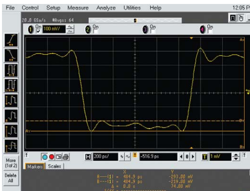
Figure 3. Ripple captured at 100 mV/div on an Agilent 54855A scope.
